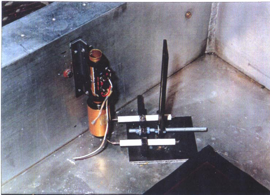
Figure 8a. Ignitor positioned below compensator.
