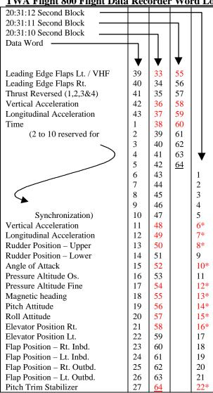
There are 43 data words recorded by the Flight Data Recorder and 64 words are recorded in sequence, each second. The chart above presents recorded data from the Flight 800
