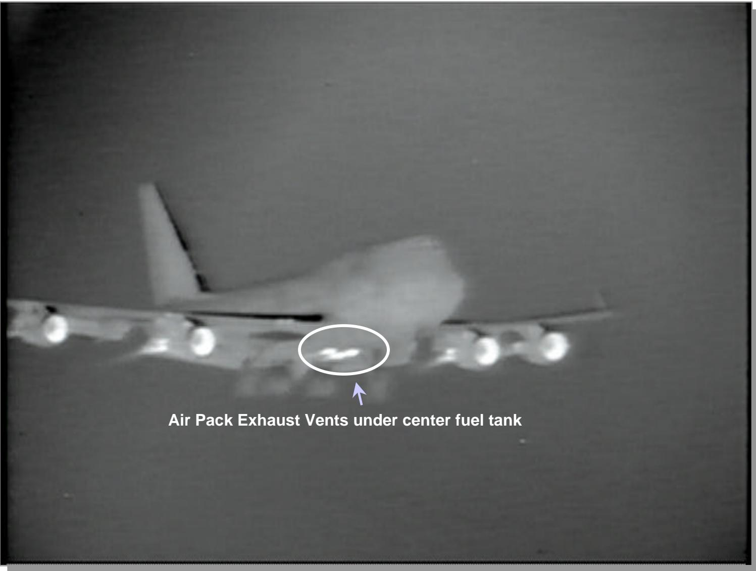
Air Pack Exhaust Vents under center fuel tank
